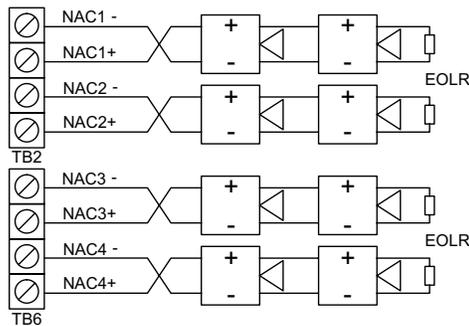
Marking indicates output signal polarity when the circuit is active. Polarity reverses when the circuit is not active. Wire notification appliances accordingly. Notification appliance polarity shown in active state.
