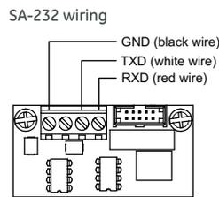
The RS-232 card is installed on the plastic assembly and connects to the main circuit board via a ribbon cable.
